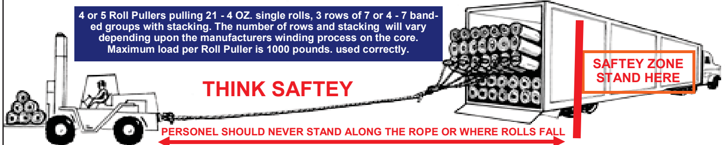
3 Roll Pullers pulling up to 12- 4 OZ stacked single rolls or 4- 5 banded groups with stacking may be possible.
